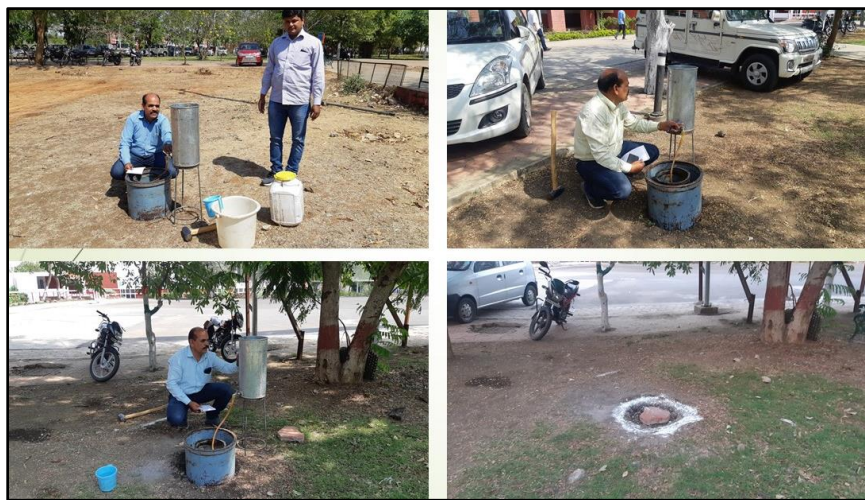
Figure 3.9: Photographs showing infiltration test
