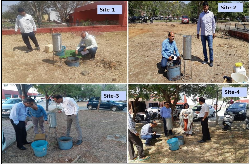
Figure 4.10: Photographs showing infiltration tests at four sites in WALMI campus
